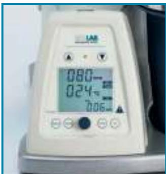
*Integrated operating panel for convenient control of the main unit and heating bath.*
