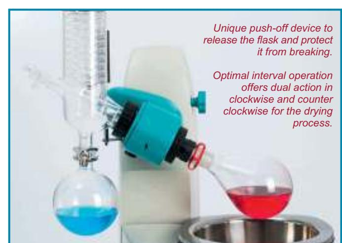
*Unique push-off device to release the flask and protect it from breaking.*
